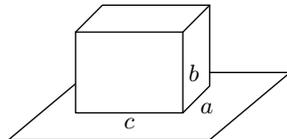
We can see that it's more efficient to turn the cuboid over one of the edges with length  $c$ , because  $a$  is shorter, so it's easier to lift the center of mass so that the cuboid would turn over the edge with length  $c$ .
