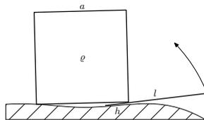
From equality of torques at the point where the crowbar touches the cube (the middle of an edge), we can find a formula relating the force  $F$  which we’re exerting on the crowbar and the force  $f$  with which the crowbar is acting on the edge of the cube
