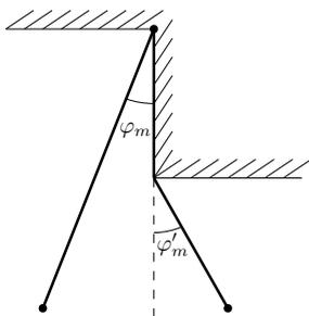
There is a pendulum, depicted schematically (with distances and angles not corresponding to this problem) in the figure. When swinging on the left side, the pendulum has length  $l$  and angular amplitude  $\varphi_m$ . On the other side, half of the rope is stopped by a wall and the remaining half swings with an angular amplitude  $\varphi'_m$ . If  $\varphi_m = 5.0^\circ$ , what is  $\varphi'_m$ ? Assume that it is an ideal mathematical pendulum without energy loss.
