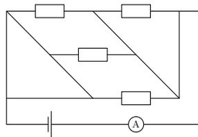
Ohm’s law says that the circuit needs to have total resistance  $\frac{2}{5}R$ , where  $R$  is the resistance of one resistor. If there are only four available resistors, the only way to achieve that is by connecting in parallel: one resistor, one resistor and two serially connected resistors. That corresponds to exactly one cut, as shown in the figure.
