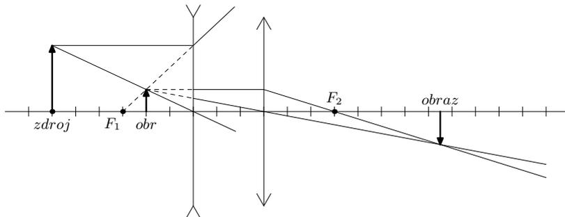
we can find out that the image will be formed 2 units of distance before the first lens (“obr”). This image will be formed 5 units of distance from the second lens, which will form it at the distance 7.5 units before itself (“obraz”).
